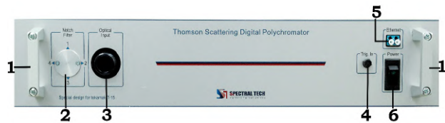
Picture 3 Digital Polychromator for Thomson Scattering. 1 - handles, 2 - notch filter for Rayleigh calibration, 3 - optical input, 4 - trigger, 5 - optical Ethernet, 6 - power switch
