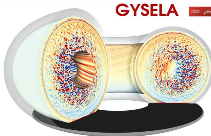
**Figure:** 3D visualization of the turbulent fluctuations of the electric potential resulting from the 5D GYSELA simulations with penalized immersed boundary.
